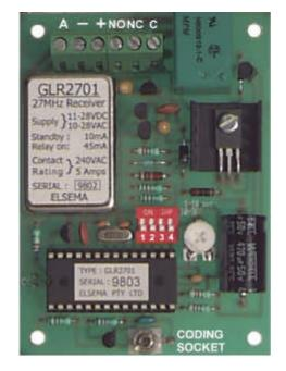
The GLR2701 microcontroller in-built code programming system automatically selects the programming mode that provides flexibility in programming the receiver channel to different transmitter channels. In programming mode the receiver sends a random code to program the transmitter channel. Momentary joining the two CC pins on the receiver board sets the channel to a random code. To program the receiver to the transmitter channel(s) follow the steps outlined in the transmitter instructions.
